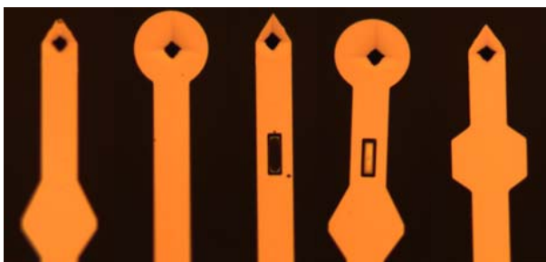
Figure 6. Geometries of some of the cantilever tailored for bimodal AFM operation. Design and manufacture by NWs.
