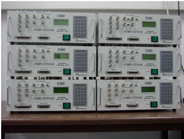
Figure 5. Picture of six of the bimodal AFM units manufactured by the CSIC and Eldisa within the ForceTool Project.
