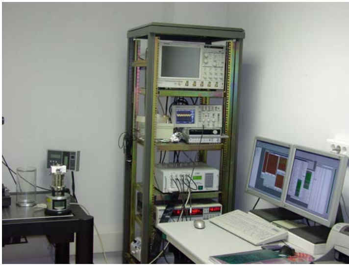
Figure 4. Bimodal AFM microscope. The instrument combines a commercial AFM platform with the bimodal AFM controller developed in the ForceTool Project.
