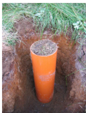
Fig. D36-7: Excavation of undisturbed soil columns in the field
