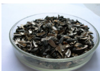
Fig. D36-11: Sorbent sunflower husks used by INMPE
