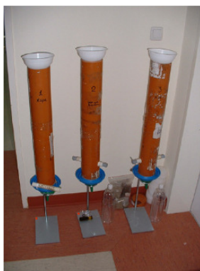
Fig. D36-8: Lab-scale soil column experiments
