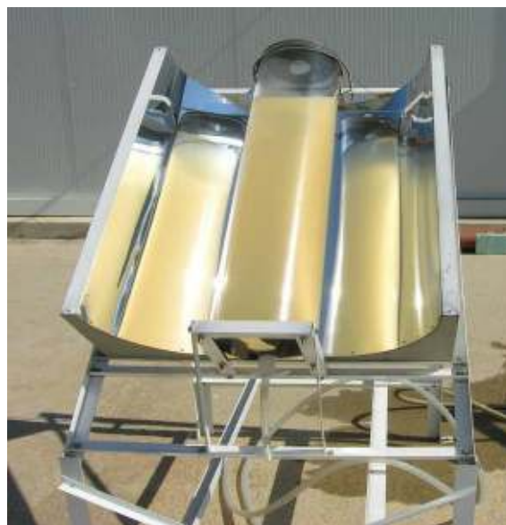
A 25 litre enhanced batch reactor fitted with a compound parabolic collector
