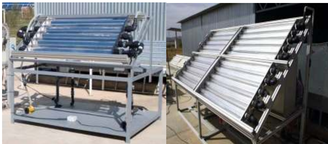
Figure 20. Picture of the 14 l-solar CPC reactor (a) and 70 l-solar CPC reactor (b) at PSA facilities (Almería, Spain).
