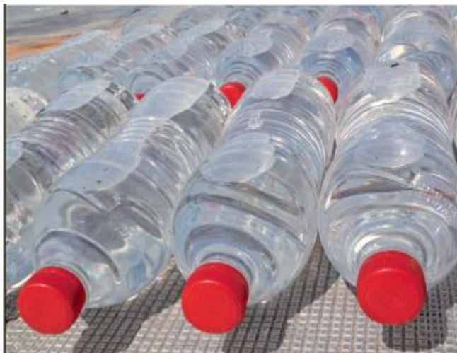
Plastic SODIS bottles filled with water and set out on the roof of the CIEMAT laboratories in Almeria Spain. Bottles were exposed over 6 months. Assays were conducted every month.
