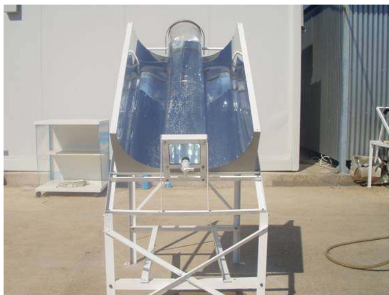
Figure 28: Batch CPC SODIS (25 L total volume).
