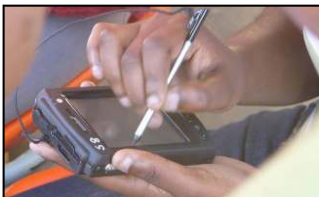
Figure 3: “Symbol Pocket PC” handheld computer used to capture field data.
