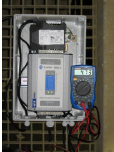
Fig. 8. Current measured at the receiver located at 50 meters from the sensor.
