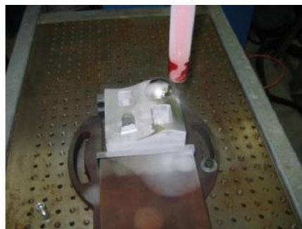
Figure 7: CO2-treatment of milled mould
