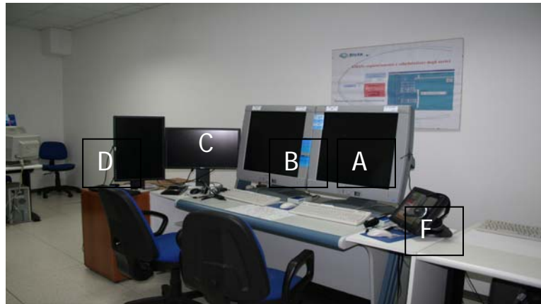
Figure 7. The executive and planner working position used during the simulation. The display were as follow: planner 2D radar display (A), executive 2D radar display (B), executive 3D radar display (C), and finally executive navigation display (D), see text for description. In front of the controller (F) was also placed the input device for the Instantaneous Self Assessment Tool for workload measurement.
