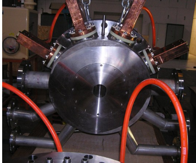
Figure 17: The SEISM 60 GHz ECR source prototype.
