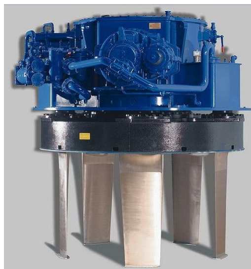
Figure 7: A Voith-Schneider propulsor
