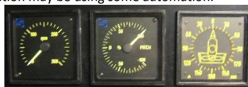
Figure 15: Triple instrument (rpm, pitch, angle)
