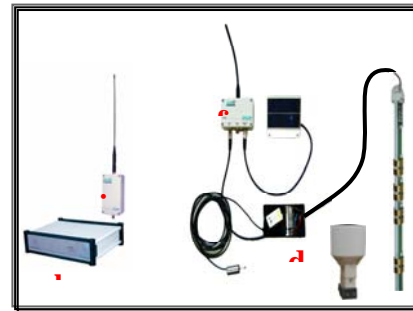
Photo 1: Components of the automatic Irrigation scheduling prototype. a) multisensor capacitance probe, b) capacitance sensor, c) LVDT sensor, d) special circuit, e) rain gauge, f) radio transmission unit RTU, g) solar panel, h) telemetry gateway, i) radio modem.
