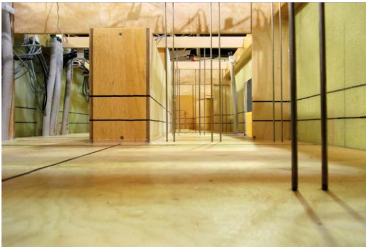
Figure 8: Vehicle deck modeling of RoPaX R2
