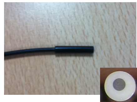
Fig.2: Fibre sensor, with cross section view (inset)
