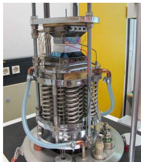
Figure 23. MTEC test-bench for module conversion efficiency available at Siemens. (Source: Siemens)
