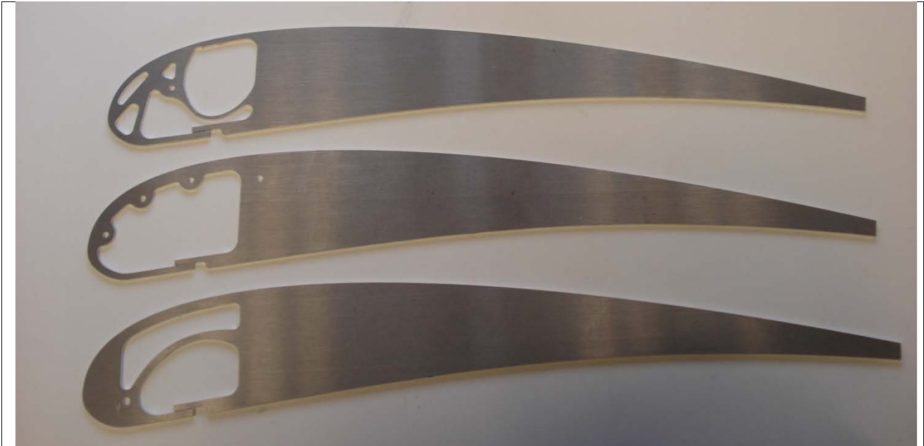
Figure 16: Various concepts of compliant leading edge concepts have been manufactured and tested.
