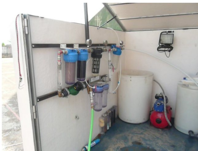
Figure 20: Photograph of the generation 1 prototype for point-of-use water treatment.
