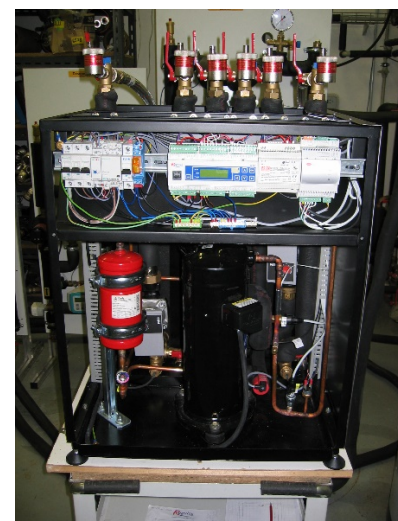
Figure 8: Hydraulic scheme and front view of heat pump that was developed by CTU & Regulus.
