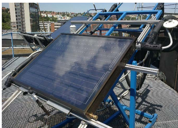
Figure 4: Glazed nonselective PVT collector at outdoor testing, glazed selective PVT collector at indoor testing.
