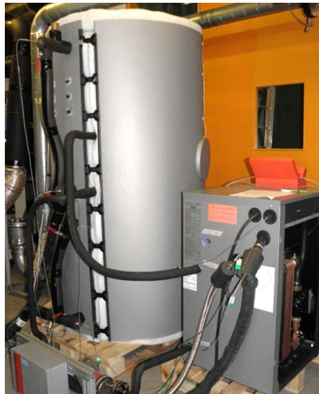
Figure 12: Storage with integrated heat pump condenser built by Viessmann & CEA INES.
