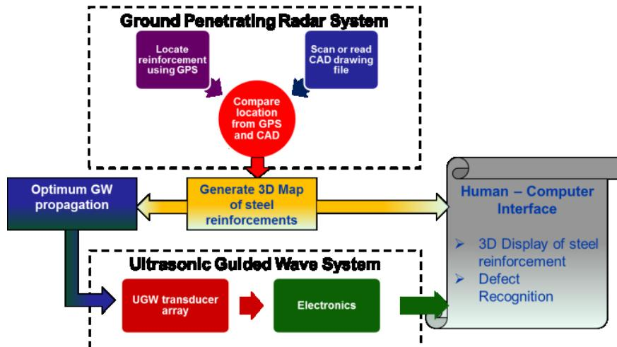
The technology is based on a hybrid system of Ground Penetrating Radar (GPR) and Ultrasonic Guided Waves (UGW), using the positioning advantages of GPR to locate the internal steel reinforcements, and UGW, to detect flaws and corrosion on those. The system will display the results as a visual 3D map on a dedicated laptop running a purpose designed program.
