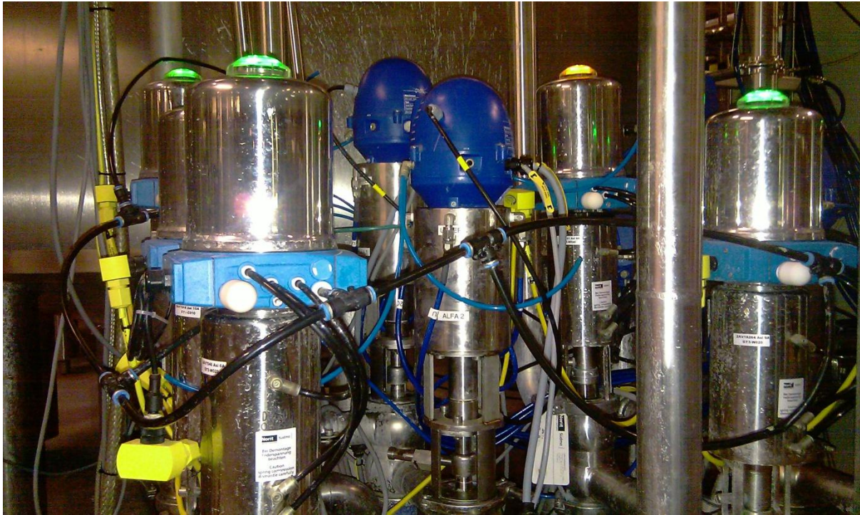
Figure 20. Pre-demonstration Hydract actuators fitted to Alfa laval valves
