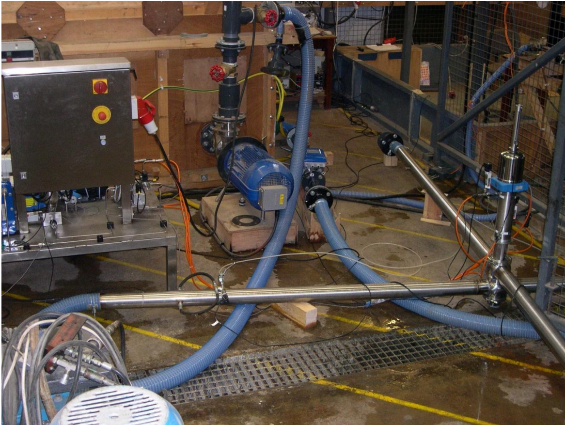
Figure 5. Flow loop used for qualification testing of actuator
