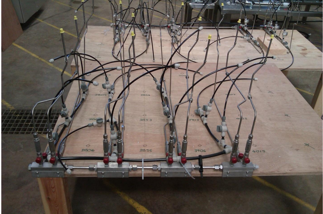
Figure 17. Mock-up of manifolds and pipework for CIP 2 valve matrix
