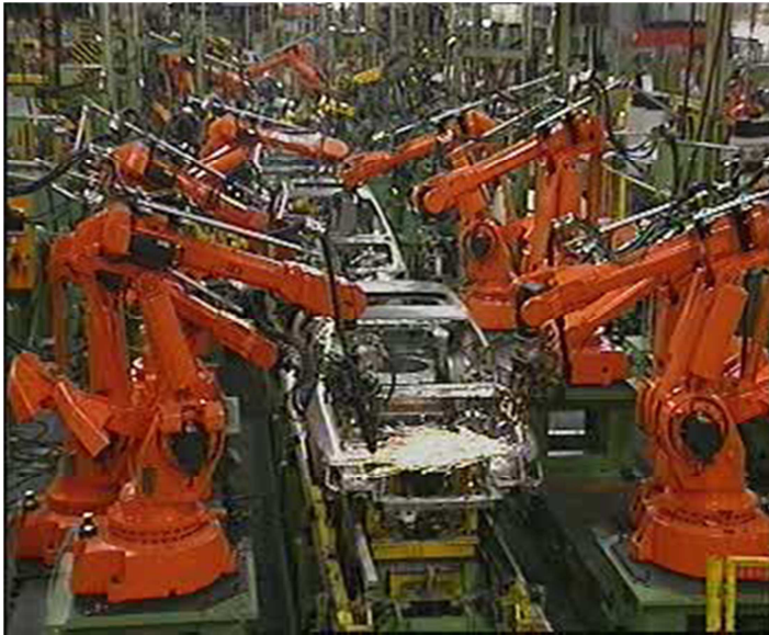
Figure 1. Automated car production employing resistance spot welding
