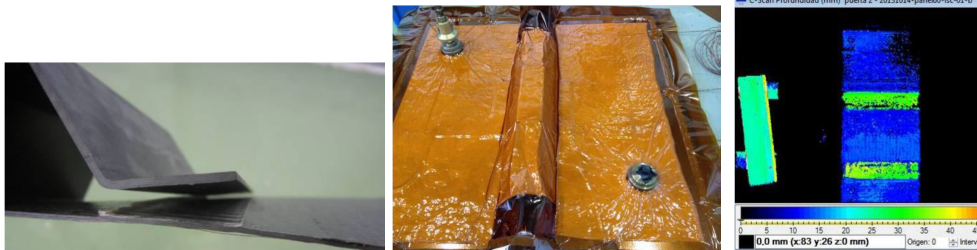
Figure 11: Final status of the demonstrator one foot unbounded (a). Post processing vacuum bag (b). C-scan of repaired demonstrator (c)
