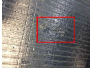
Figure 10: Repaired no consolidated tow
