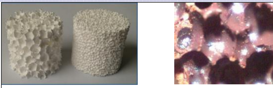
Figure_ 6 30 and 45 ppi foams; optical microscopy
