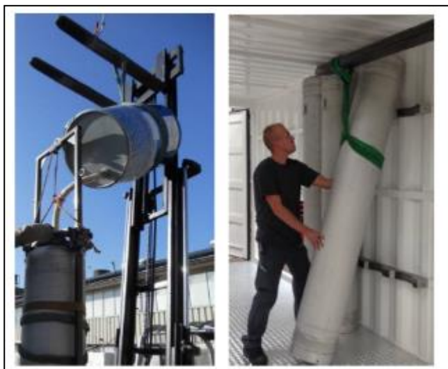
Figure_ 8 Filling of PSA vessel with PSA adsorbent material (left) and its installation in the PPS housing (right)
