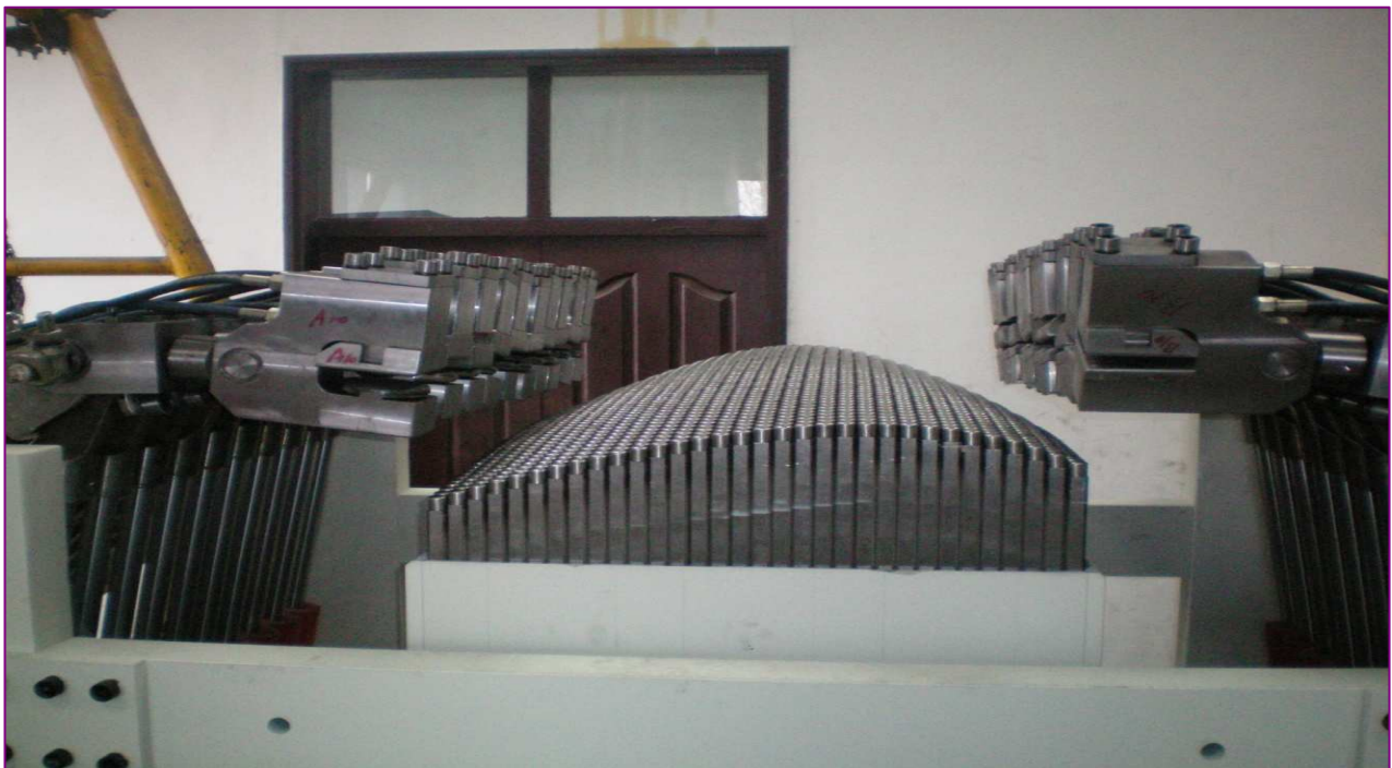
Fig. 2 MPSF tooling and new stretch machine built by JLU
