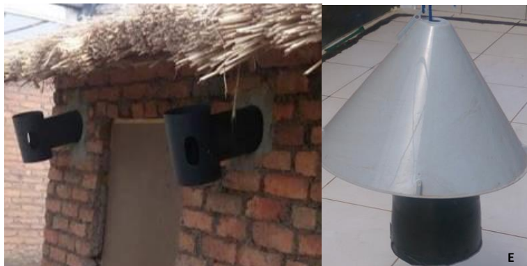
Fig. 7. Left: Outdoor host-seeking prototype devices attached to eave tubes inside a semi-field system brick house. Right: bottom-entry design of a stand-alone OHD with conical cover.
