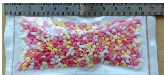
Fig. 4. Permeable membrane pouch containing slow-release polymer granules loaded with three different attractive components.
