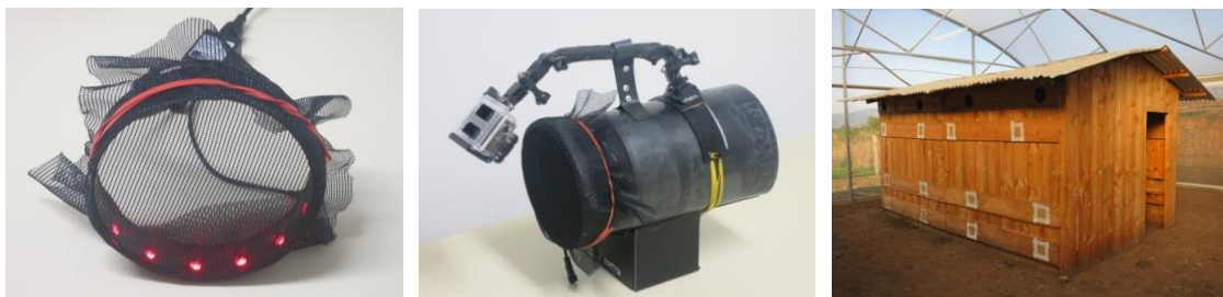
Fig. 9. LED light source (left) fitted on an eave tube with mounted GoPro camera (middle); experimental hut in semi-field system for video studies (right).
