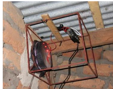
Fig. 13. Videoing of wild mosquitoes entering the Eave tube and contacting the netting in Sagamaganga, Tanzania.
