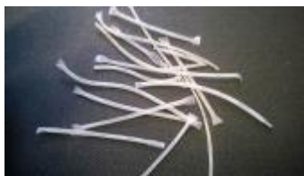
Figure 16 – Example of hollow fibre capsules. Length of these fibres was about 20 mm.
