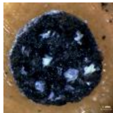
Figure 7 – Impregnated lightweight aggregate. The white spots are the healing agent inside the pores of the particle.
