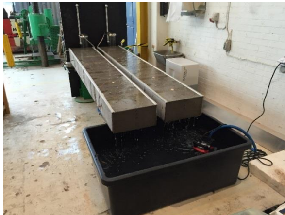
Figure 31 – Set-up for exposure of the beams to water/NaCl solution.
