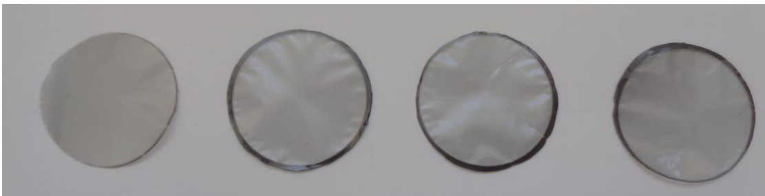
Figure 2: Optimized dispersion of graphene compounds (compression moulded discs)
