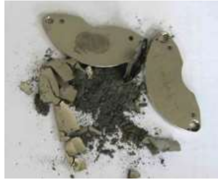
HD VCM magnet showing the large pieces of Ni
