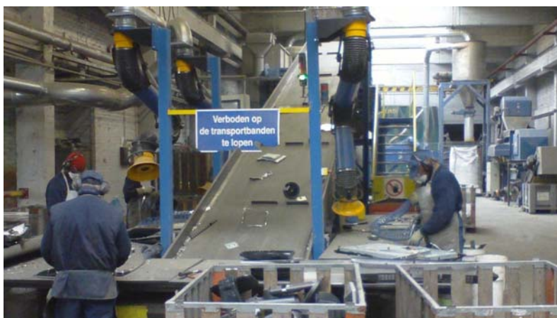
Figure 1. FPDs recycling line, pre-disassembly operations
