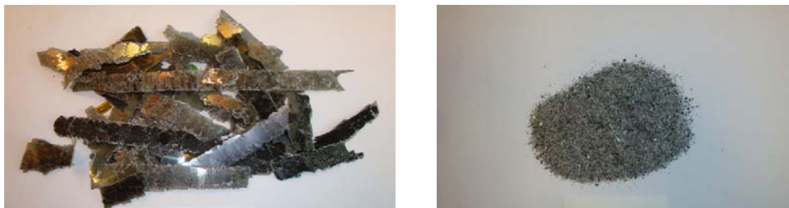
Figure 2. Output fractions after first shredding step
