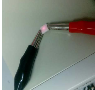
Figure . Encapsulation of \text{Y}_2\text{O}_3:\text{Eu}^{+3} phosphor in LED lighting
