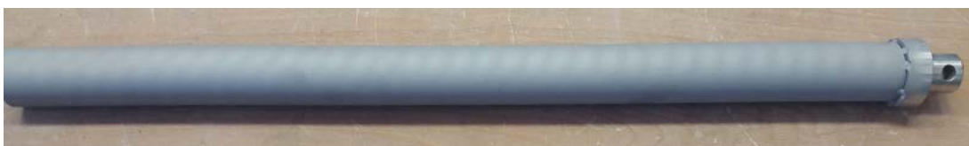
Fig. 25. P92 tube coated externally by CoNiCrAlY (HVOF).
