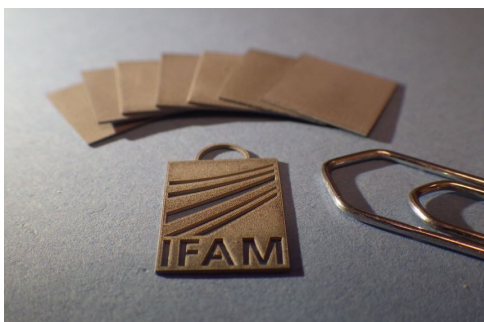
Figure 3.8: Plates of La-Fe-Co-Si prepared with the first binder recipe.
