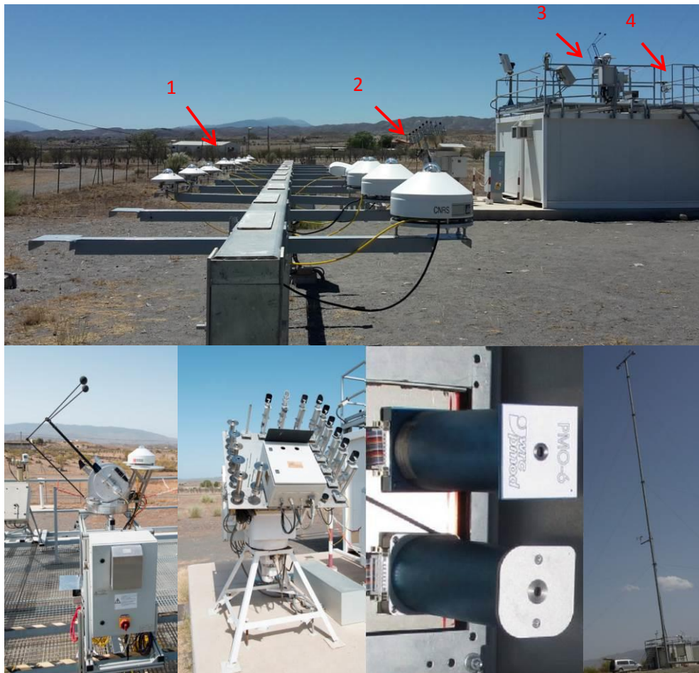
Figure 13. Top: Overview of Metas calibration setup (1: Pyranometer test bench; 2: Pyrhemometers test bench; 3: Black Photon tracker with DHI reference; 4: cloud camera); Bottom left: detail view of Black Photon tracker; Bottom left centre: detail view of pyrhemometer test bench; Bottom right centre: two absolute cavity reference pyrhemometers located in the pyrhemometer test bench's front cabinet; Bottom right: Metas wind mast.
