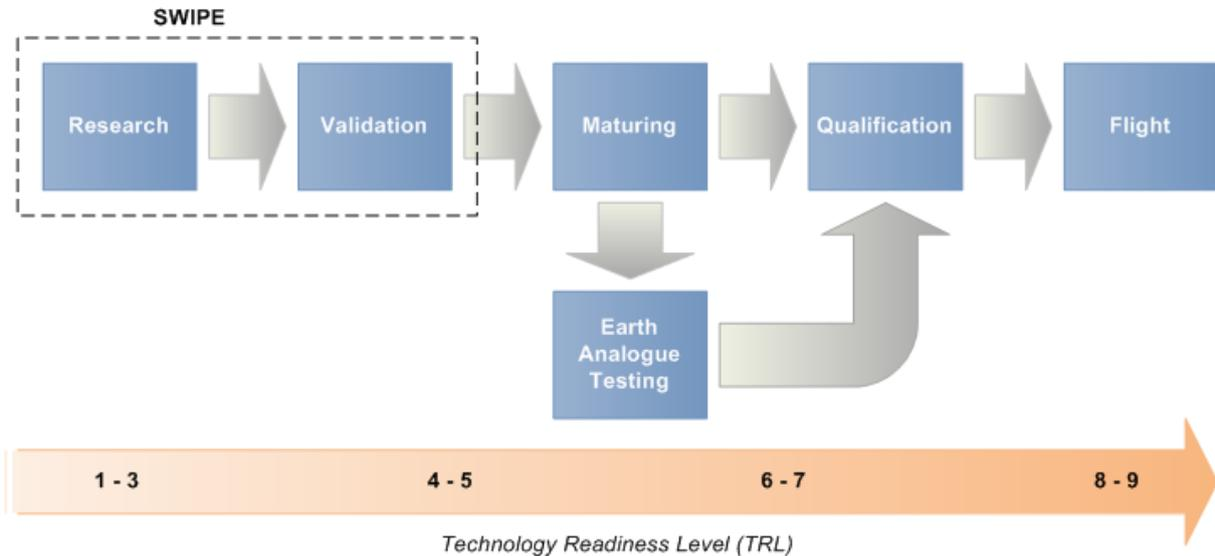
**Figure 5 – Typical space technology evolution and development phases.**
