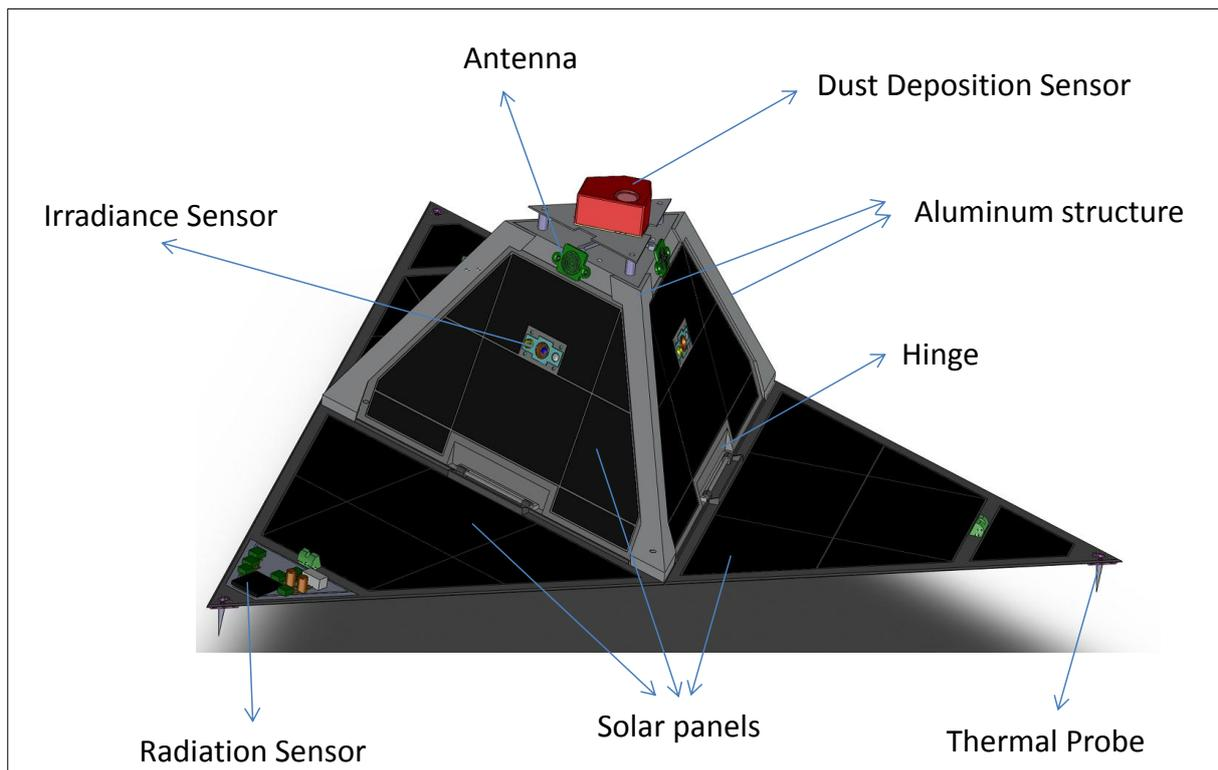
**Figure 4 – SWIPE node configuration (open, after deploying panels).**
