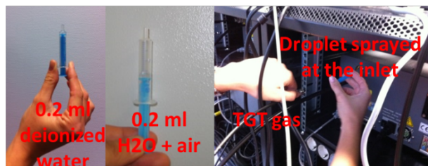
Figure 5: Protocol of the water vapor correction assessment with droplet method.
