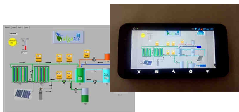
Fig 7. Details of control system and monitoring screen in Smart-phone with remote control of inoculum production plant.
