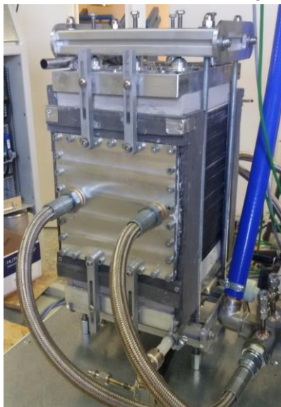
Figure 14. The graphite resin based Demstack HT PEMFC stack of 1kW power.
