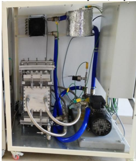
Figure 16. Integrated stand alone HTPEMFC stack system of 1kW power.
