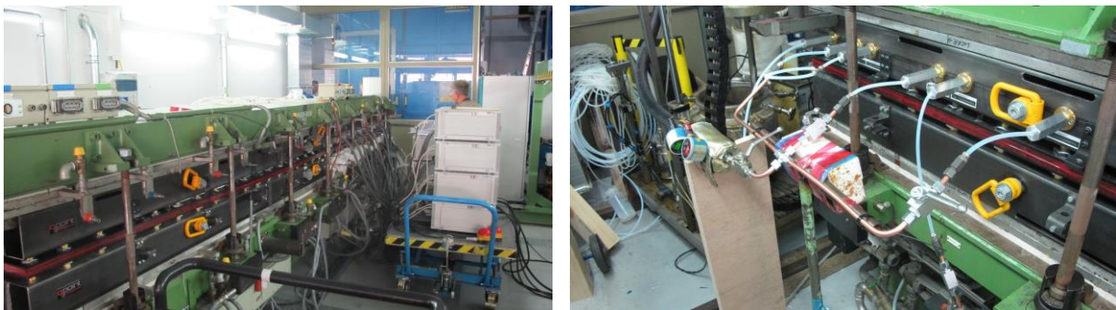
Figure 13 Closed mold with the controllers (left), resin inlet ports connected to the inject. device (right).
