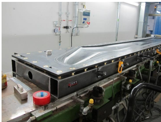
Figure 10: Manufactured set of CFRP RTM tools with integrated heating.
