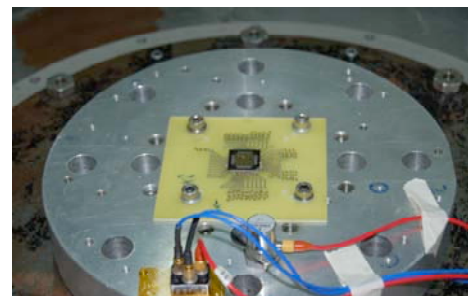
Fig. 5. PCB with the SENPIMAG sensor fixed on the sample holder for the vibration test
