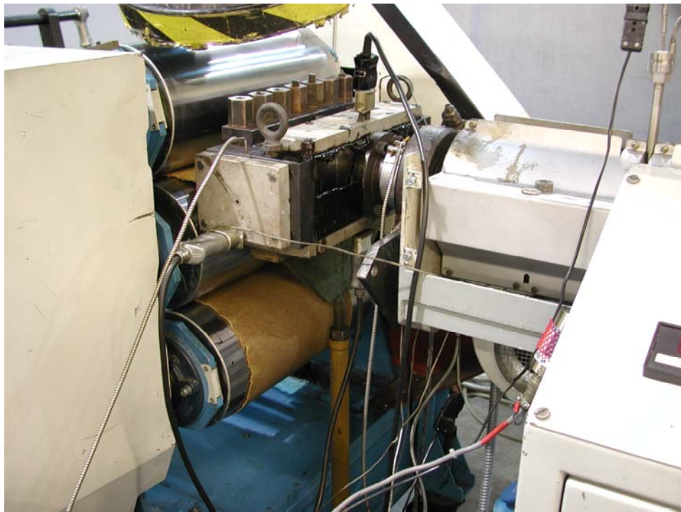
Figure 4: Pilot Natural Fibre Sheet Production
