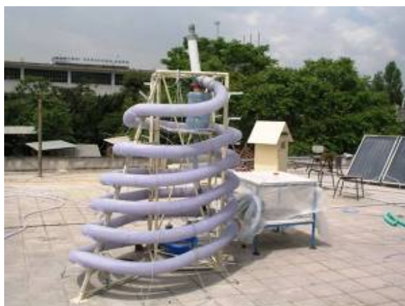
Design and construction of the pilot-scale boa photobioreactor
