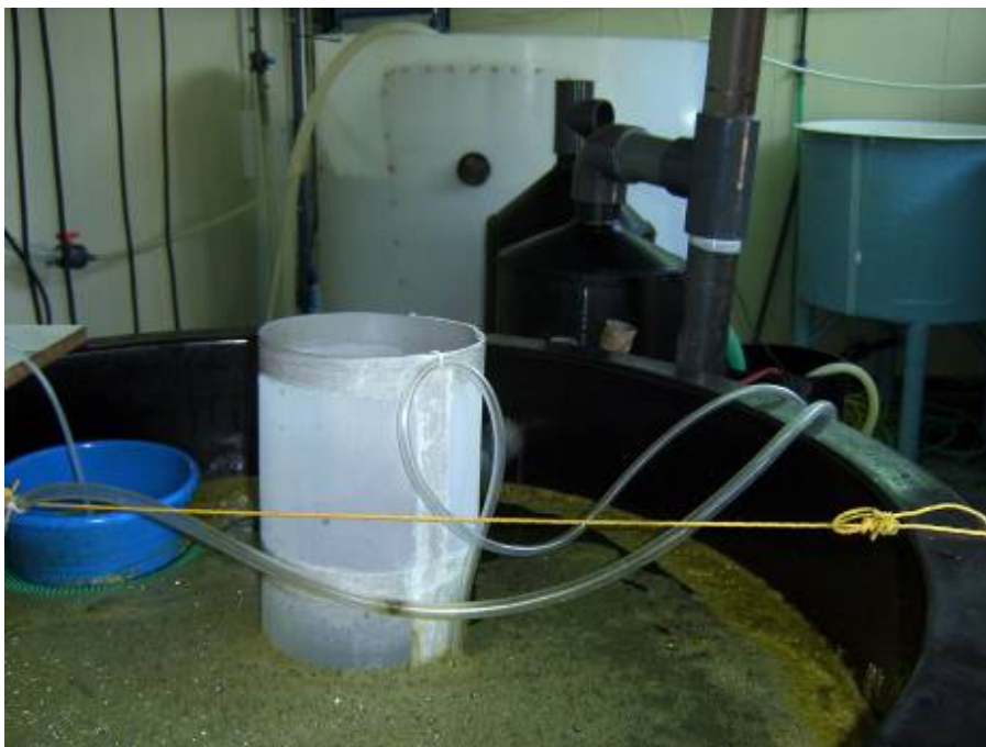
Rotifer tank with flock trap and internal filter
