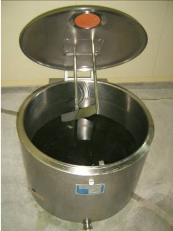
300 liter milk chiller installed at Argosaronikos with concentrated algae.
