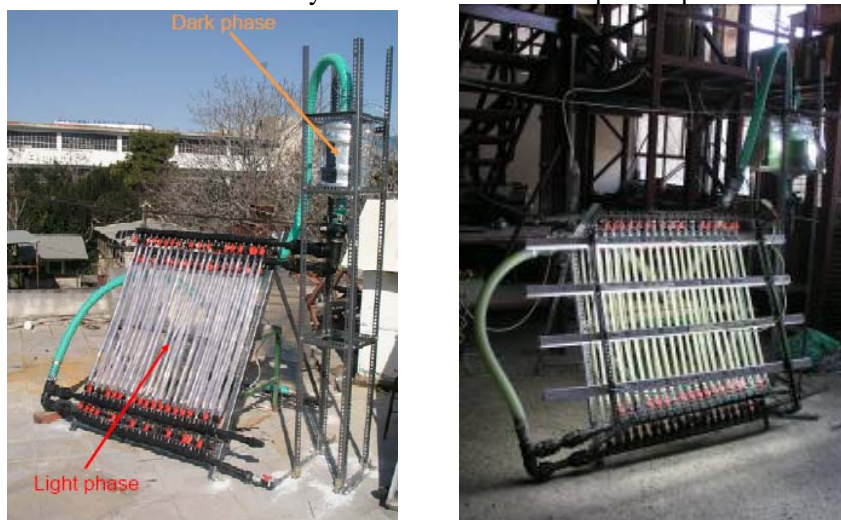
Design and testing of the thin tube bioreactor outdoors and indoors with artificial lights
