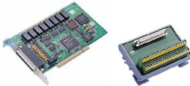
Figure 12: Pictures of the PCI Relay card and the wiring terminal for this card
