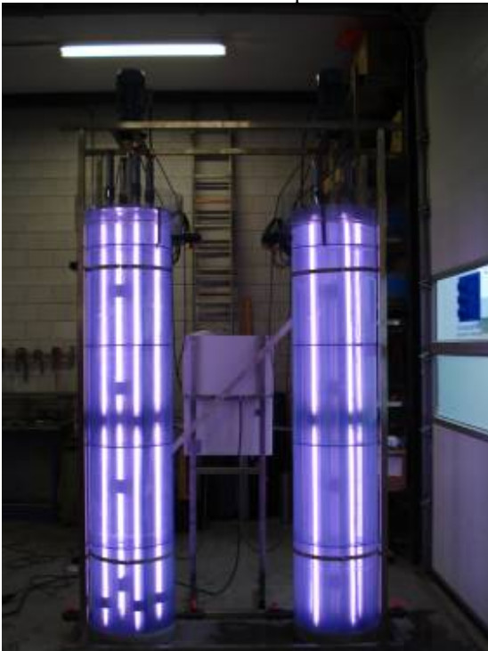
Double photobioreactor with and with out internal lights on
