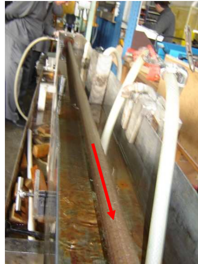
Bio Shelter product running through the water bath having exited the calibrator
