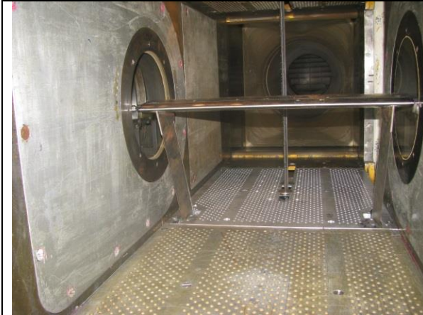
Figure 1. T-112 TsAGI transonic wind tunnel with installed wing model and pylons for compressed air supply.
