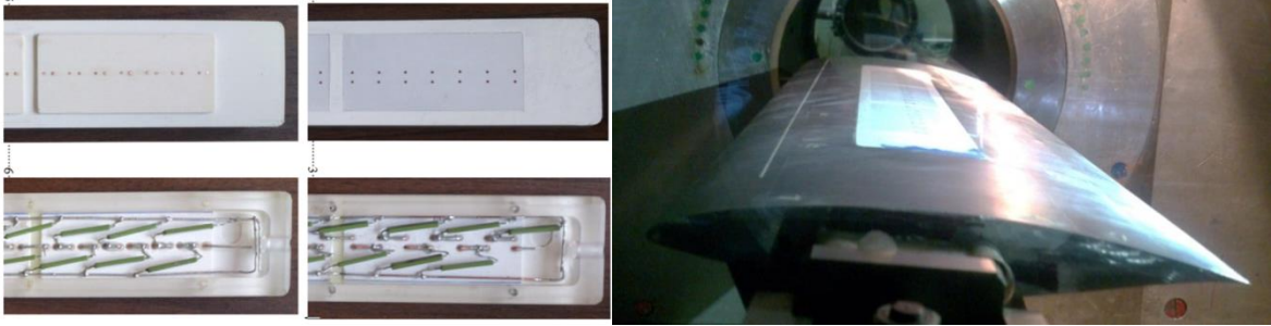
Figure 12. Two inserts and wing model with spark actuator installed in TsAGI T-112 WT.
