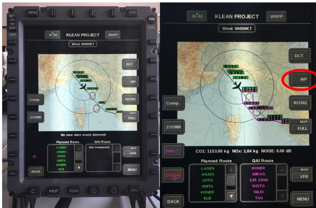
Figure 27: The GUI main screen soon after the no flight zone event on the left, and on the right presentation of routes and waypoints. Planned route and its waypoints are all in green, the Q-AI proposed route and its waypoints are in magenta. The WP button switches on/off the visibility of labels.
