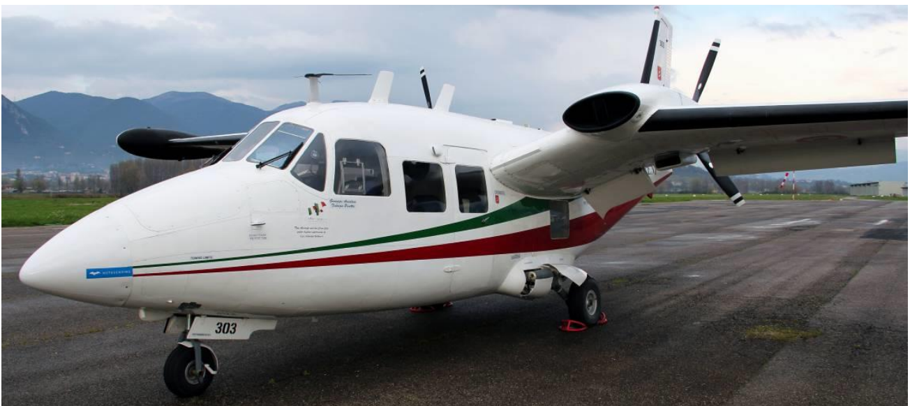
Figure 11: Nose pod-equipped P-166 at the airport of Terni (IT) during the second XWALD measurement campaign.
