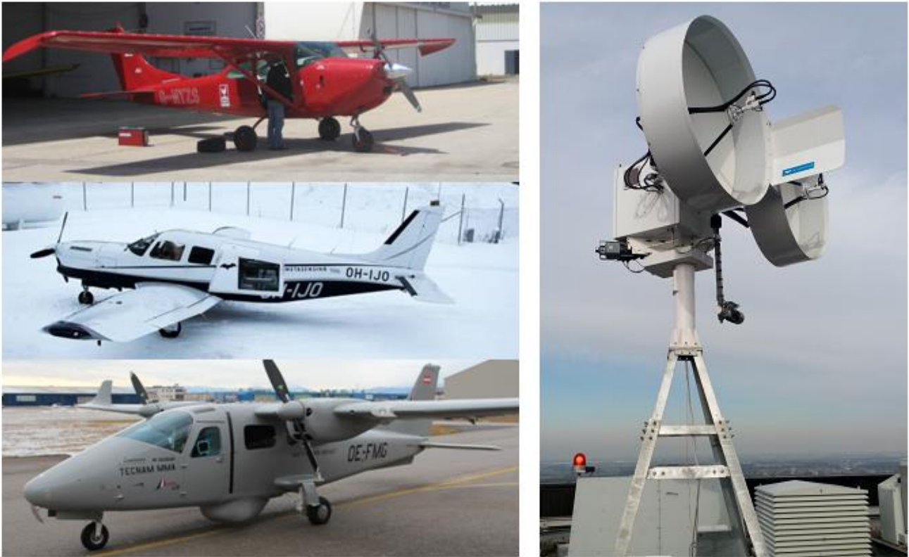
Figure 2: Examples of experience by MetaSensing in radar design and deployment: on the left, a number of aircraft platforms used in different radar acquisition campaigns performed at X-band. On the right, the MetaXWR X weather radar installed on top of a high building in Rotterdam (NL).
