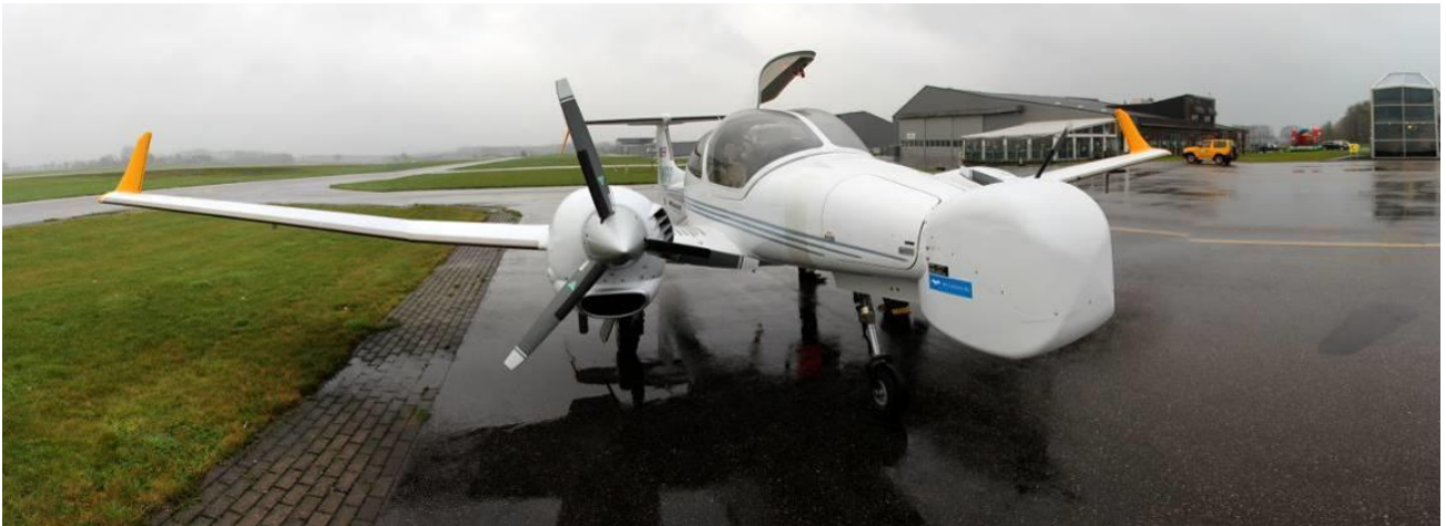
Figure 10: Nose pod-equipped DA42 at the airport of Teuge (NL) during the first XWALD measurement campaign.
