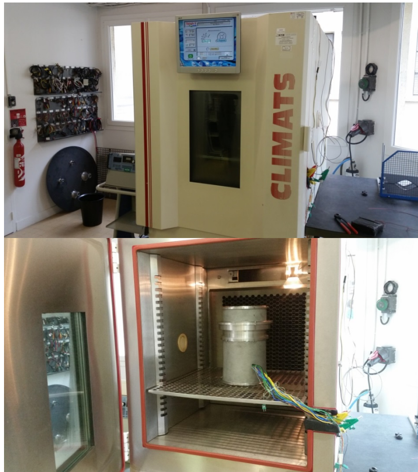
Figure 25 – LMB environmental test chamber to conduct the high temperature tests required within EFFAN. In the picture below we can see the EFFAN fan prototype ready for testing
