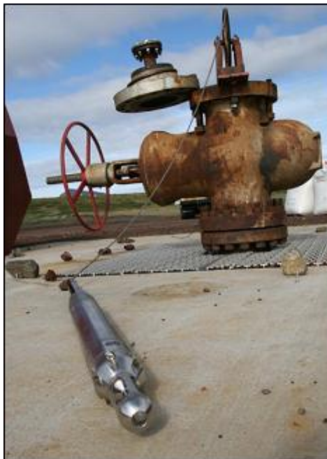
Figure 4: BRGM temperature tool before going into a high temperature well at Krafla.
