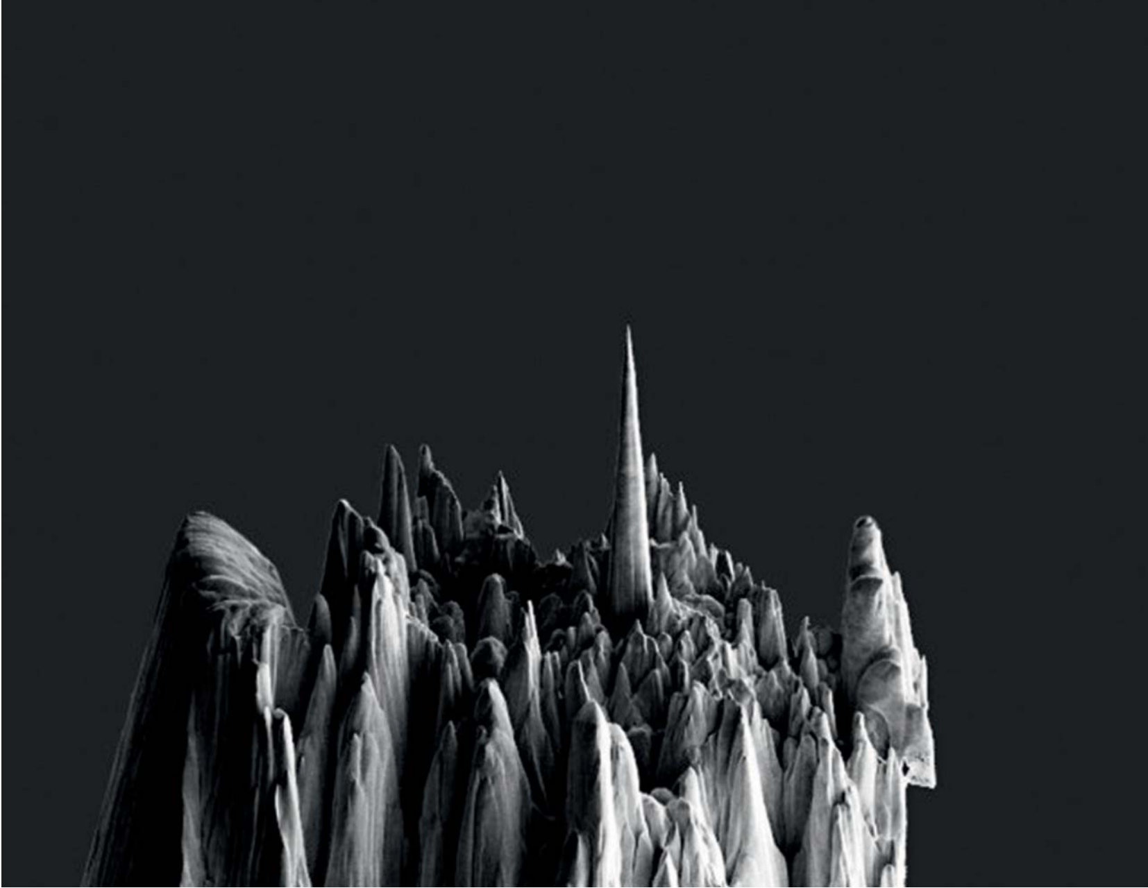
Tip of a Scanning tunneling microscope (STM), sharpened by focused ion beam milling down to an apex size of few tens of nanometers. Experiment: G. C. Gazzadi, V. Corradini, S3 (INFN-CNR) Modena; Artwork: Lucia Covi. ©S3.
