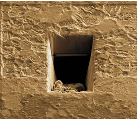
Micrometric trench in a multilayer material formed by copper, silicon oxide, silicon, obtained through focused ion beam (FIB) milling. Experiment: G. C. Gazzadi, S. Frabboni, S3 (INFN-CNR) Modena; Artwork: Lucia Covi. ©S3
