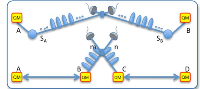
The QuReP Quantum Repeater technology is centred around quantum light-matter interactions at the quantum level in ensembles of rare earth ions frozen in a crystal that store quantum information by coherent control of the quantum degrees of freedom.
