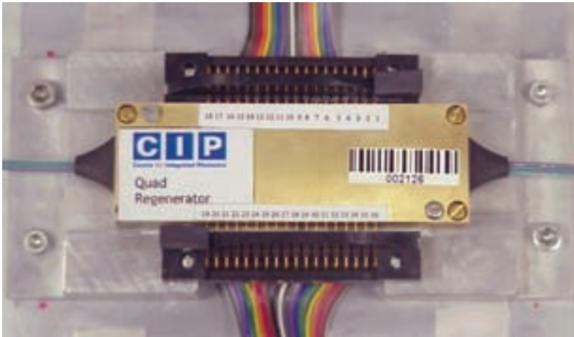
Figure 1: Fully packaged and pigtailed, 4-element, 40 Gb/s MUFINS array, using hybrid integration
