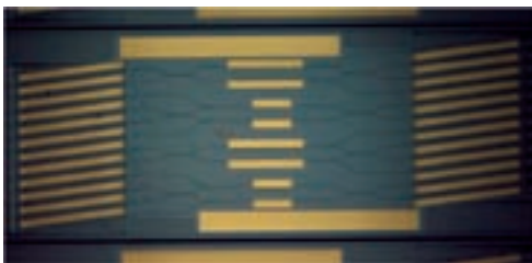
Figure 3: 4-element, monolithically integrated MUFINS device, using the active/passive integration technique based on regrowth
