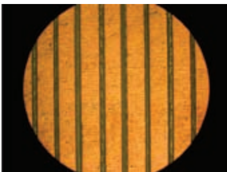
Metallic film on polymer patterned with ultrashort fiber laser
