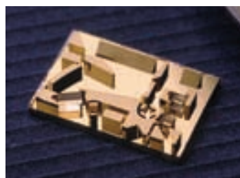
Fig. 1: The micro-optical elements for the NEMO's Educational kit 'Learn and Teach Optics' are replicated with Hot Embossing technology.
