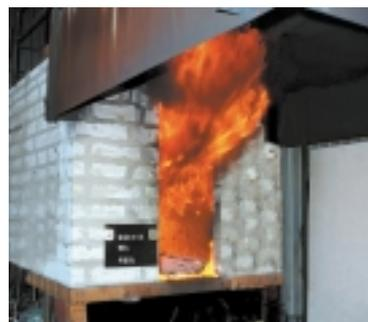
In order to solve this problem, the FIPEC project developed new small-scale and large-scale test methods for the measuring the fire performance of electric cables. The test methods developed are based on
