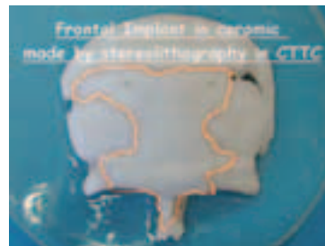
Ceramic frontal implant made by stereolithography.
