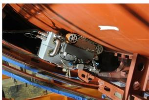
Robots take over hull inspection on ships
