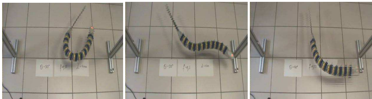
Figure 2: Experiments for tuning phase lag, resonance frequency and stationary travelling performances.
