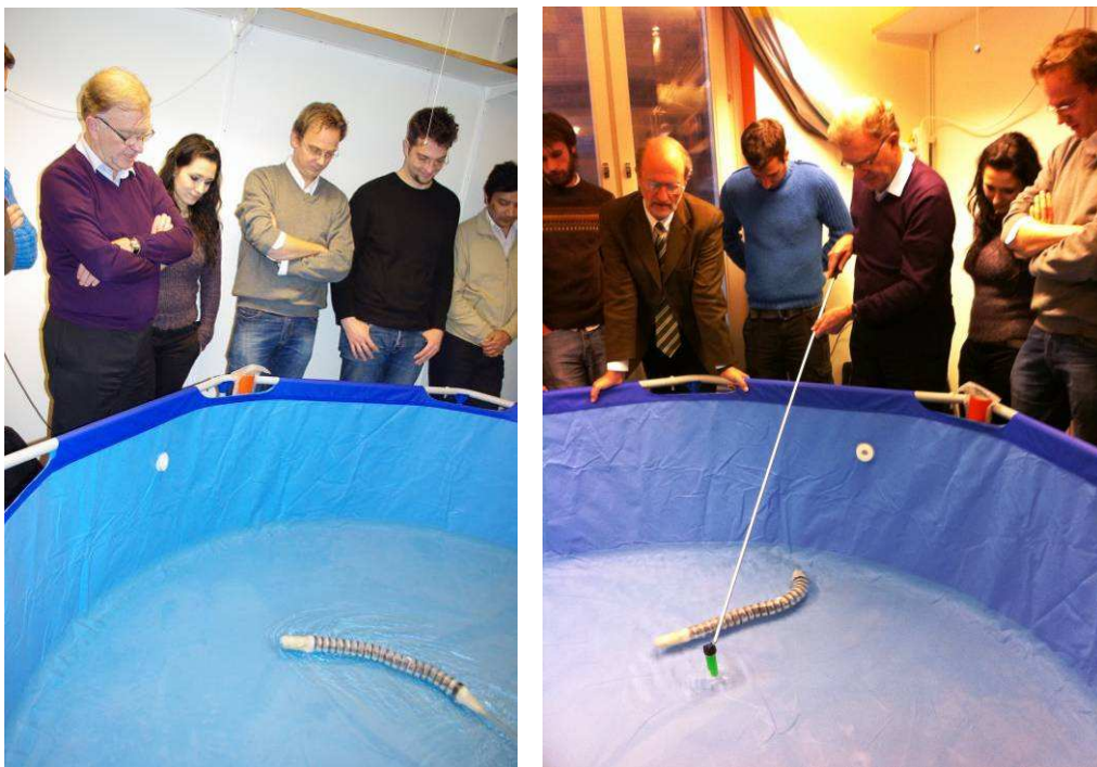
Figure 1: February 2011, LAMPETRA SSSA group; experiment at the KI. Experiments on vision system, object tracking and free swimming.
