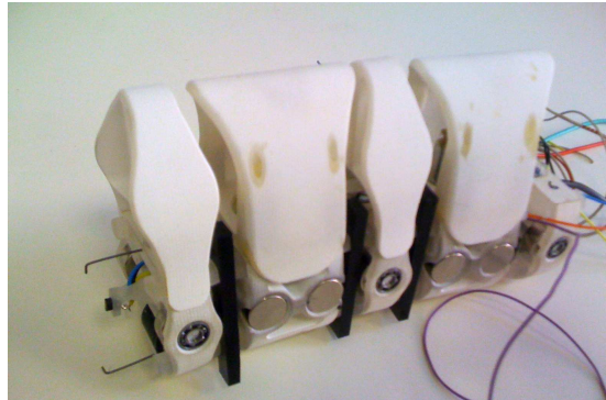
Figure 10: New vertebrae assembling for the 3D swimming robotic lamprey artefact
