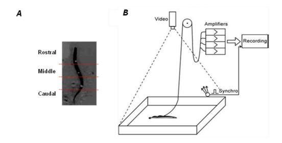
**Figure 1**. Experimental setup. A: a lamprey specimen before experiment. The red dotted lines indicate the position of electrodes implantation. B: arrangement for parallel recording of kinematical and electromyographic (EMG) data. Video- and EMG recordings were synchronized by light and electrical pulses recorded simultaneously by the 2 systems (Synchro). (modified from Islam et al. 2006)
